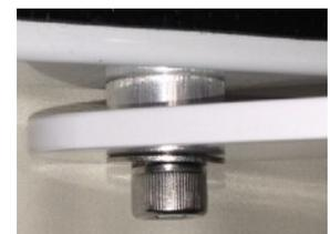
as shown. From the underside of the step place a washer and then the nut on the bolt and tighten slightly. Repeat this for the other three – A - locations.
